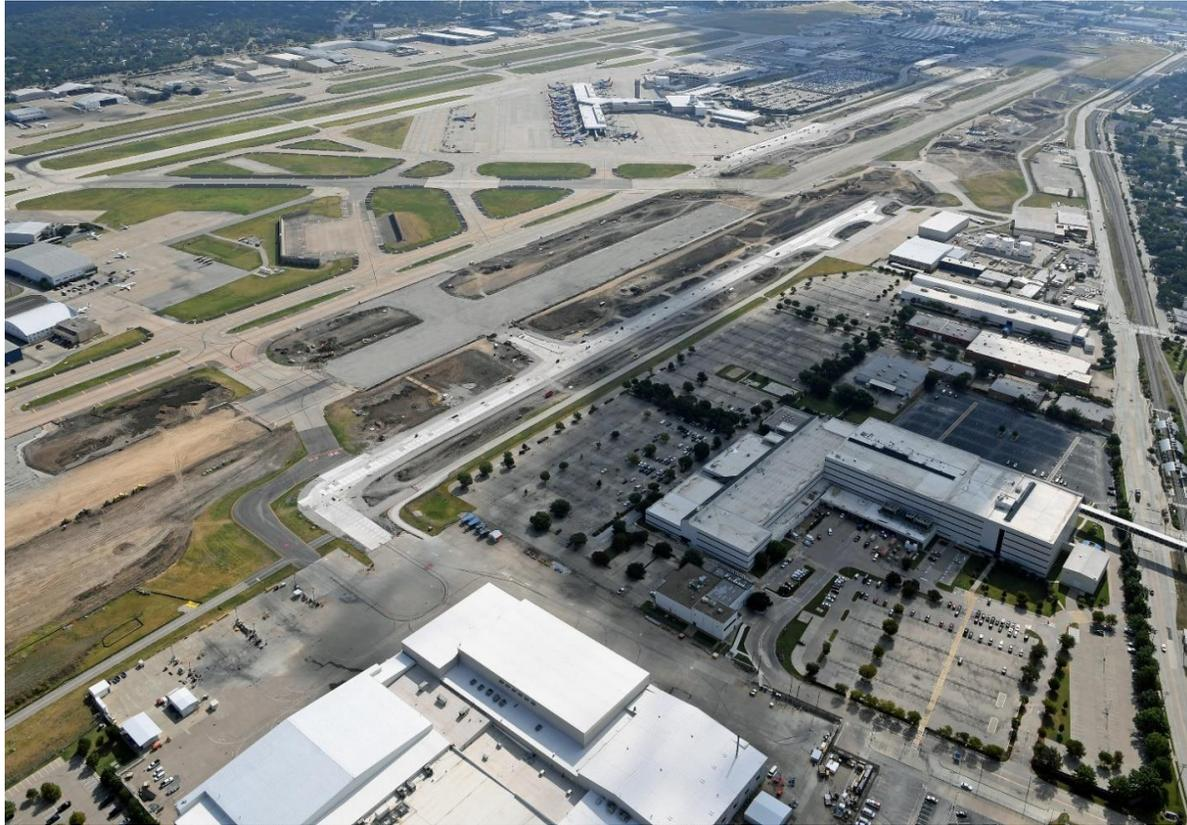
*Figure 3 - New TWY T under construction (Phase 1) and north half of RWY 13R/31L under construction (Phase 2)*
